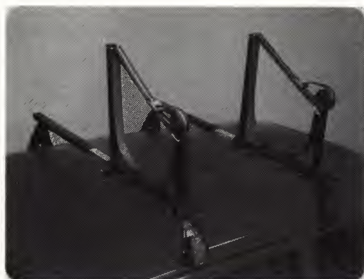
ART NO 000875 KAYAK. Kayak carrier unit. Solid galvanised steel construction in black epoxy finish. Suitable for all 20 x 30 mm cross-section bar carriers. Quick release mounting. Own weight 3.5 kg.
