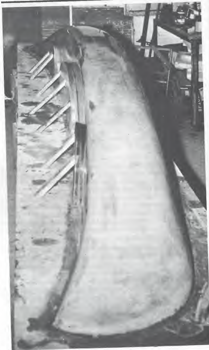
The pattern of the Cargo Slalom, ready for laying up the first half mould.
