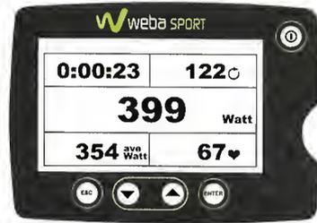
The Weba Kayak Ergo accurately measures your power in Watts, shows you your stroke length on each side and illustrates your stroke profile with a graph allowing you to identify and tackle technical issues.
