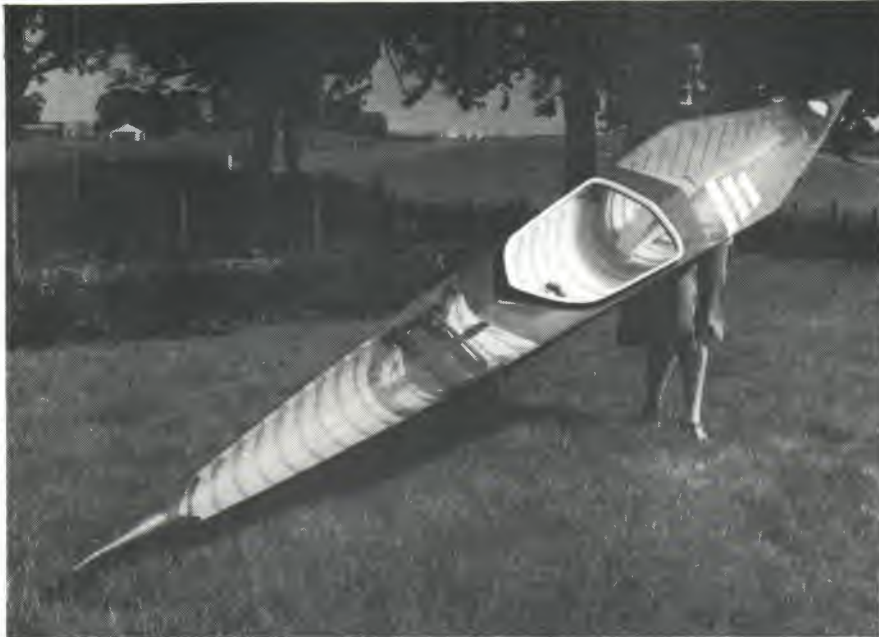
Cockpit area showing ribbed thermoplastic inner hull.
