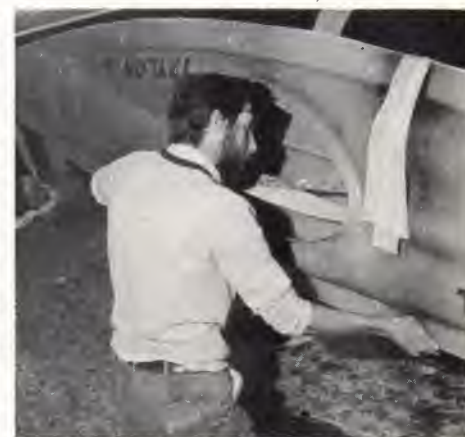
Glassing gunwale joint
