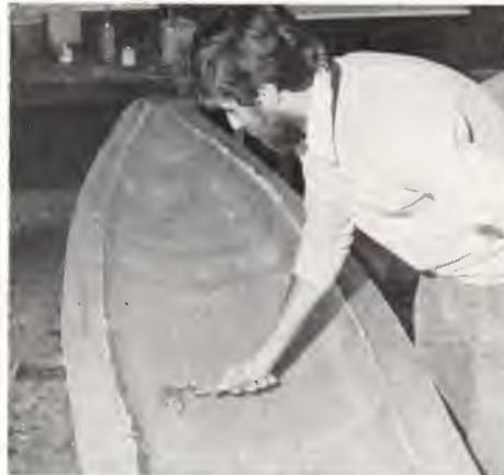
Using paddle roller on diolene
