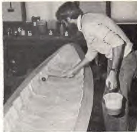
Mohair roller used on initial lay-up
