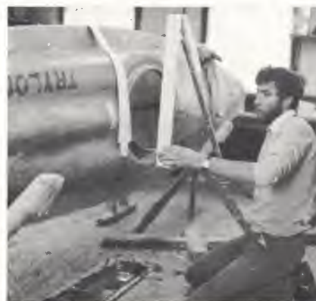
Positioning joining strip on baton
