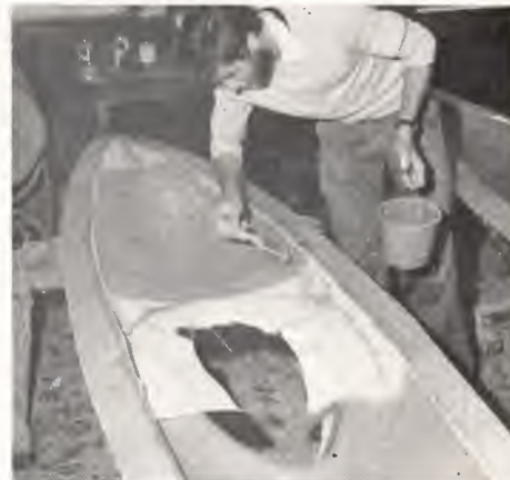
Deck lay-up showing cockpit overlap
