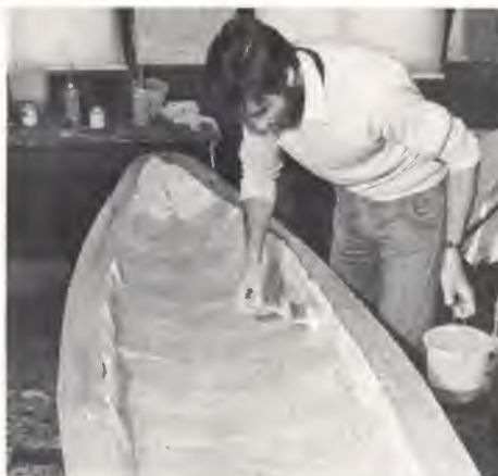
Brushing upper edges of hull mould
