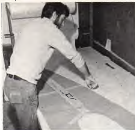
Cutting chopped strand mat to patterns
