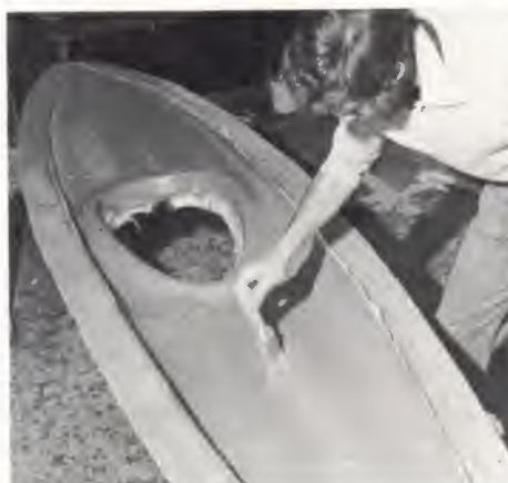
Laying-up strengthening strip on deck
