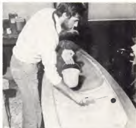
Laying-up strengthening panel
