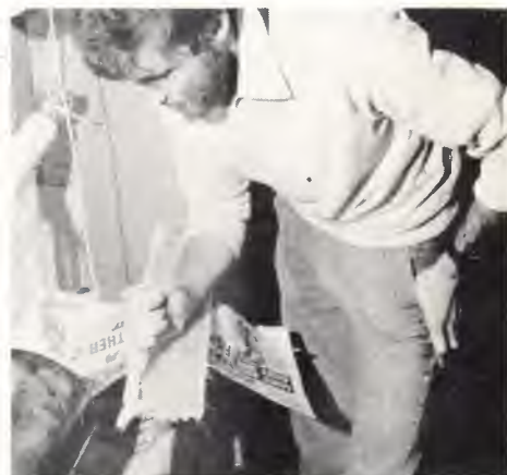
Trimming footrest lamination
