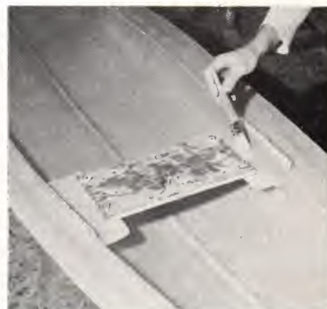
Footrests glassed in using template
