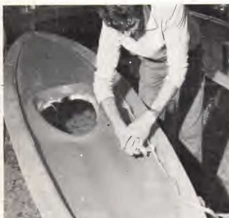
Trimming deck mould at 'green-stage'
