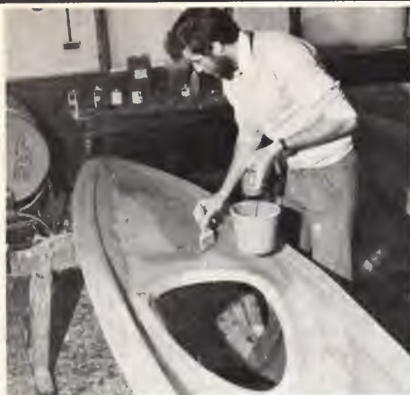
Gelcoating deck mould
