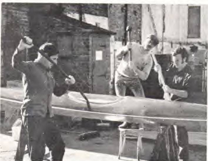
gently ease the kayak from mould!
