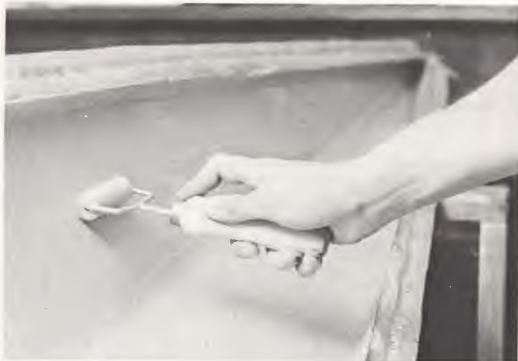
Left: The first piece of glassfibre laid in the mould and pushed down with brush. Below: Use of roller to impregnate resins through glassfibre. And trimming of waste material from mould - note cutting to outside.
