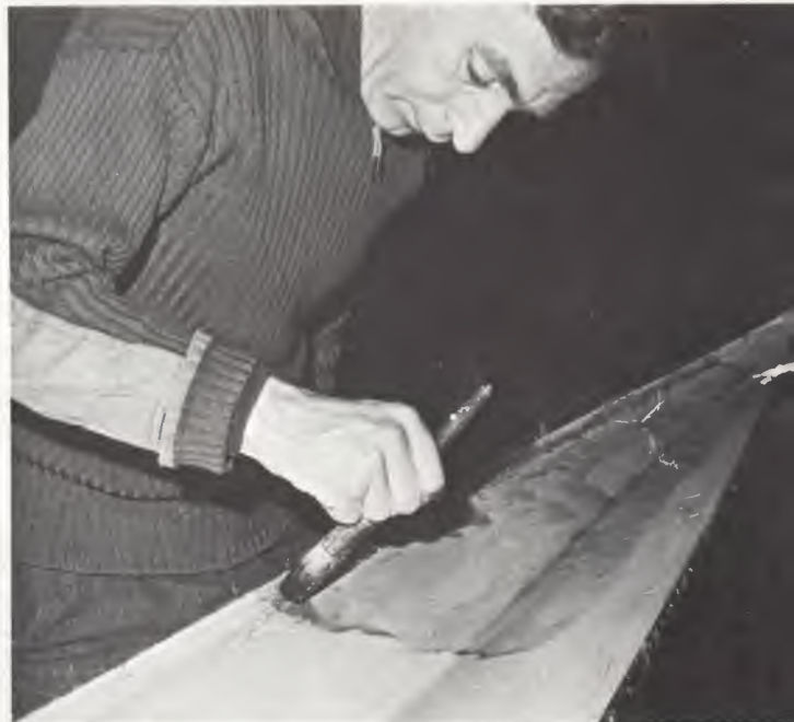
Above: The resin being applied to mould ready for the first piece of glassfibre to be laid.
