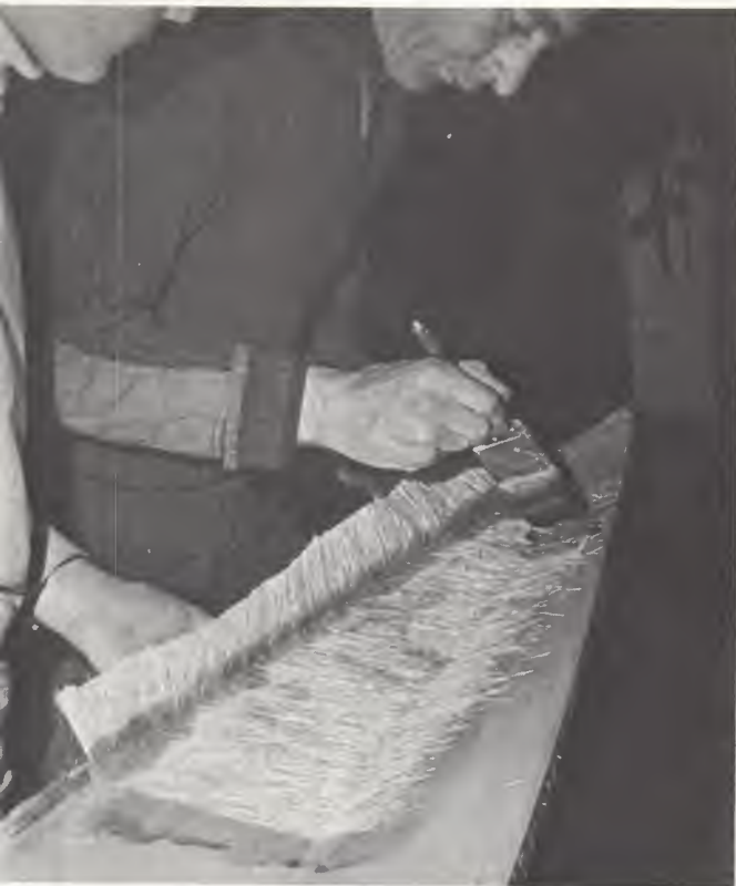
Left: The first piece of glassfibre laid in the mould and pushed down with brush. Below: Use of roller to impregnate resins through glassfibre. And trimming of waste material from mould - note cutting to outside.
