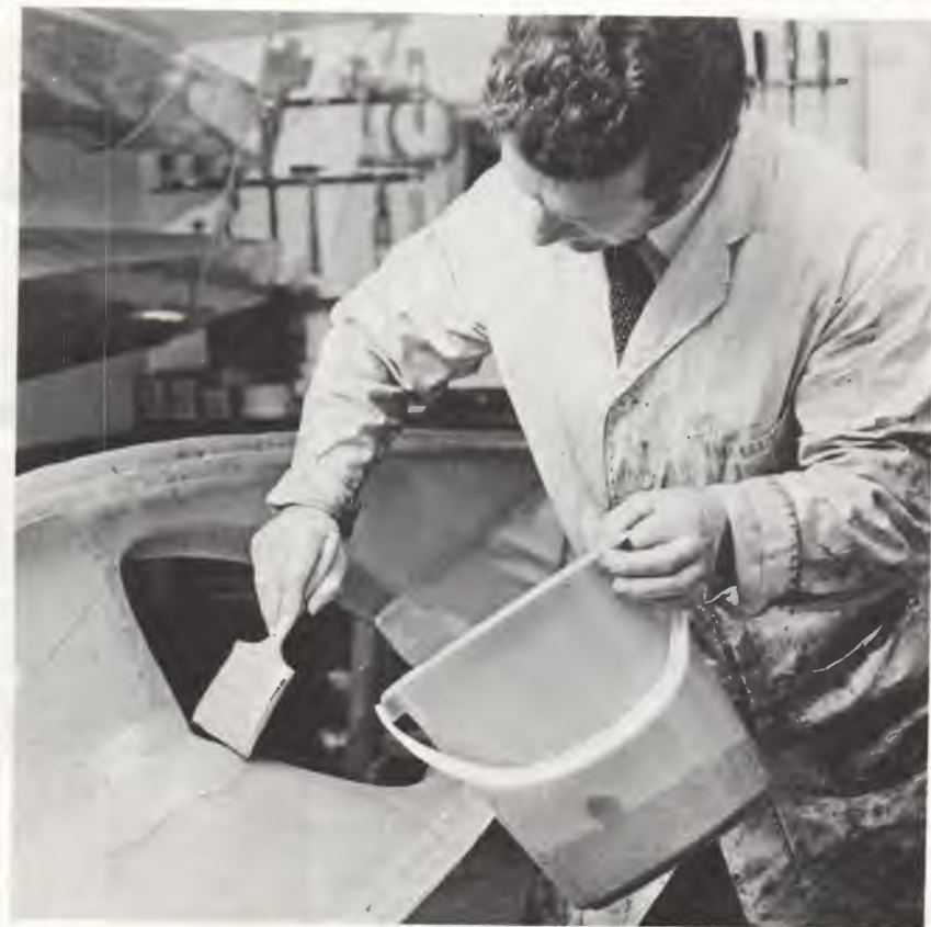
Left: Gel Coat being applied to deck mould. A liberal covering without too much worry of brush marks, providing the complete area is covered. Below: Glassfibre being cut to shapes to fit the mould.
