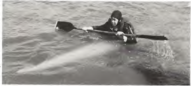
Martin Pike testing the buoyancy of a polyethylene Kayak
