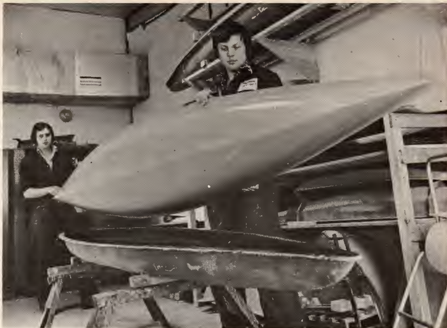
Trainees take finished hull from kayak mould.
