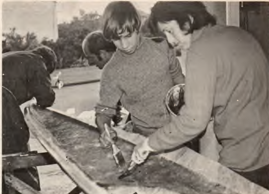
Young workers stubbing down glassfibre mat onto resin whilst making deck half of a G.R.P. canoe during a C.A.N.I. Building Course.
