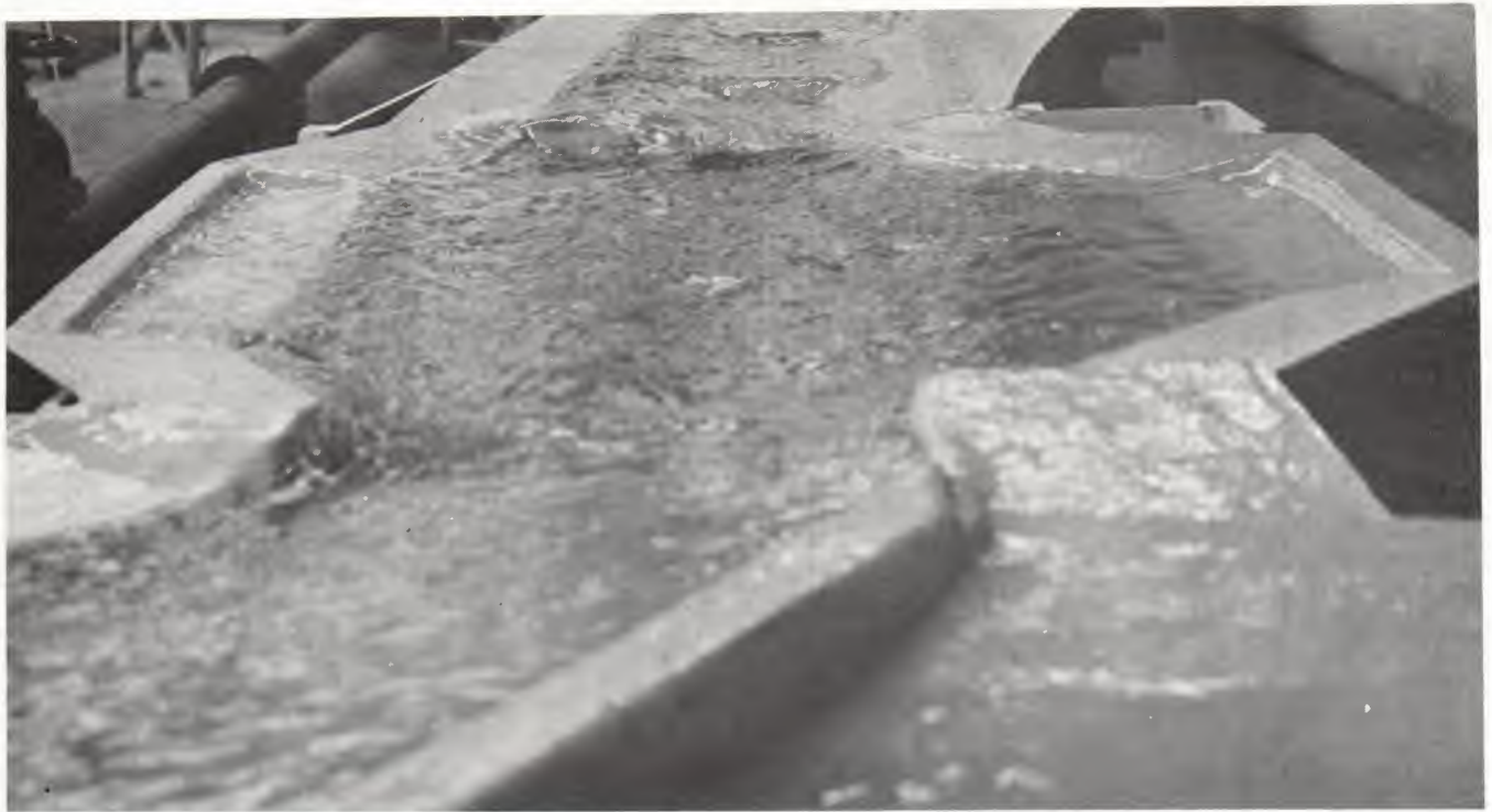
The model of the proposed slalom course, showing a succession of standing waves up to 4 feet high on the actual course.
