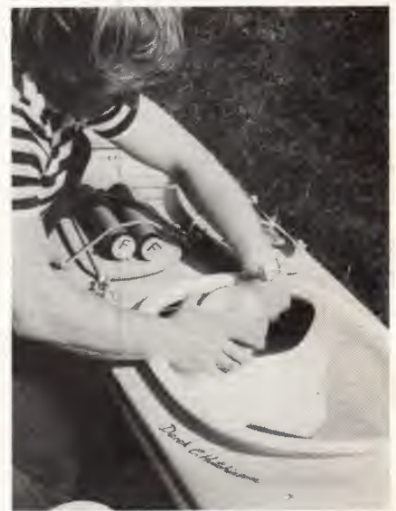
7. First aid equipment goes in the waterproof screw-top plastic container, marked with a red cross. This fits in space behind seat.
