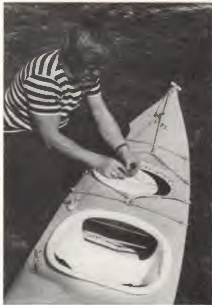
2. Circular hatch cover is secured to kayak with string to prevent loss, and is locked down. Goodies inside, not required during journey, are protected from contact with evil waves.
