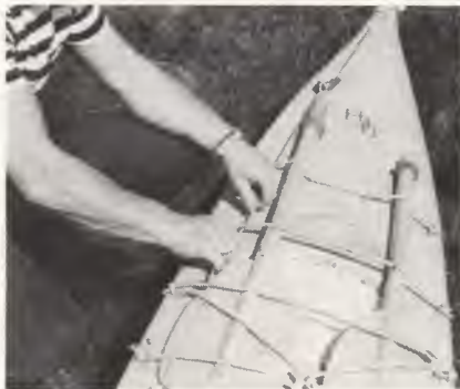
4. Tow line (which can be seen attached to stern and coiled round cleat near cockpit) is adjusted over the top of the spare paddles for easy access.
