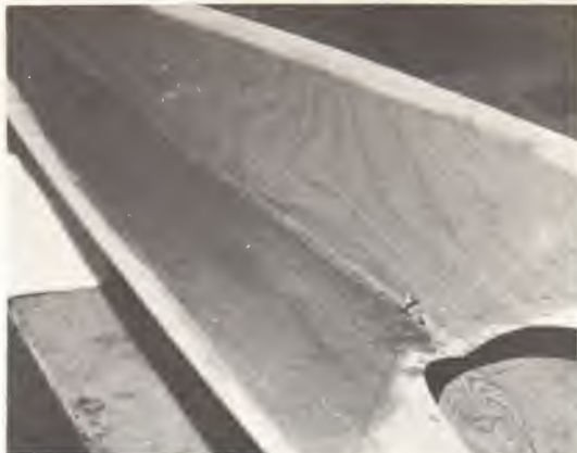
24. Deck panels complete and varnished.
