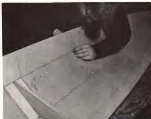
10. Lacing up the chine panels.
