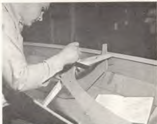
14. Fixing the cockpit frames.
