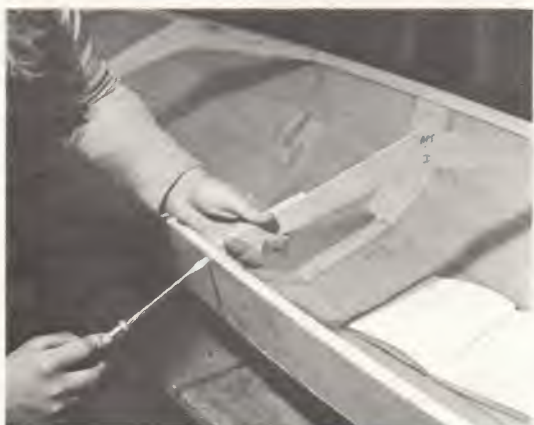
13. Fixing the deckbeams.
