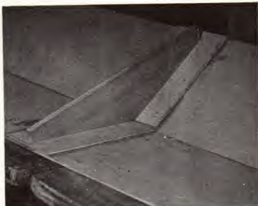
8. Temporary keel frame in position.
