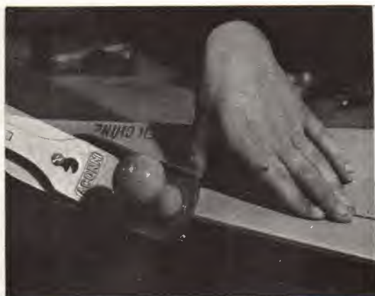
9. Bevelling the bottom panels.
