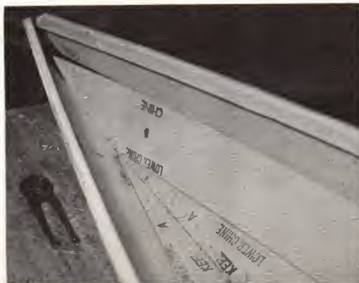
12. Laced up hull before inwales are 15 trimmed.
