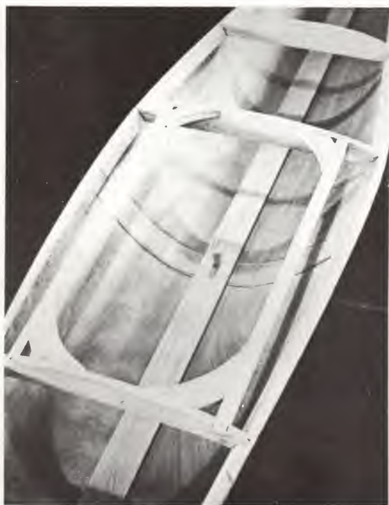
Top: Completed "Pacer" from stem. Left: Cockpit framing. Note peg on which seat fits, another is provided for the footrest. Also lap inside scarf joint. Right: From the bows. Centre two frames fitted.
