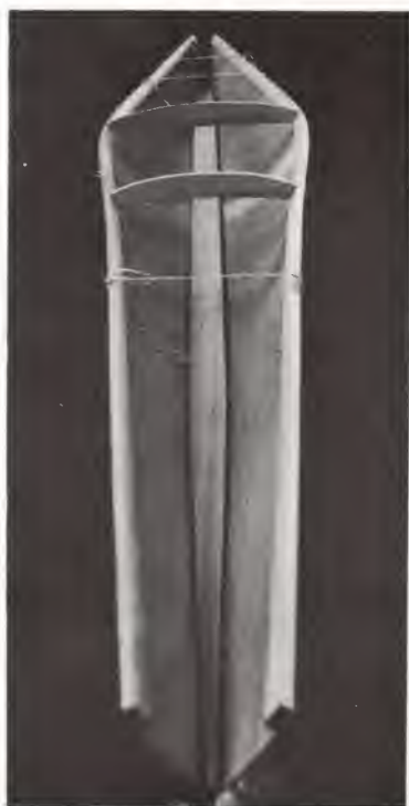
Top: Completed "Pacer" from stem. Left: Cockpit framing. Note peg on which seat fits, another is provided for the footrest. Also lap inside scarf joint. Right: From the bows. Centre two frames fitted.
