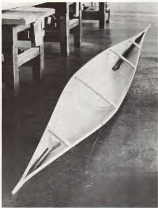
Interior from stern with four beams fitted.
