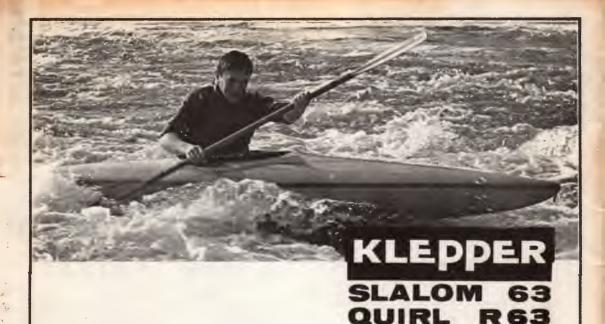
THE SLALOM '63. Moulded in glass-reinforced-plastic the Slalom '63 is the most efficient pure slalom kayak yet designed. The completely rounded cross-section gives maximum manoeuvrability and ease of rolling. Supplied complete, with built-in positive buoyancy, fixed moulded seat, adjustable foot-rest and knee-grips.
