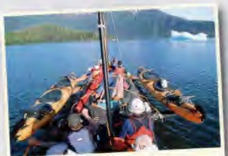
The Spirit Dancer Canoe is seen here in full expedition mode. The double Kayaks provide stability in poor conditions and the complete spray deck helps shelter the paddlers from spray and rain.
