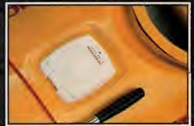
Recessed Compac 50 deck pump.
