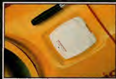
Recessed Compac 50 deck pump.
