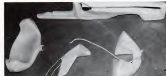
The front bulkhead, footrest, seat and detachable skeg
