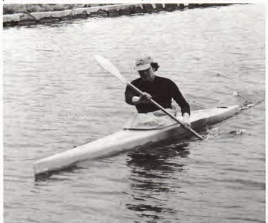
The Carbocraft K1 — one of the new breed of honeycomb aluminium boats. Pyranha plan to introduce K2 and K4 versions later in the year.
