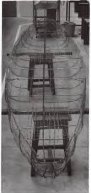
Where it all began. The steel rod and mesh frame of one of the Trent Poly concrete canoes.
