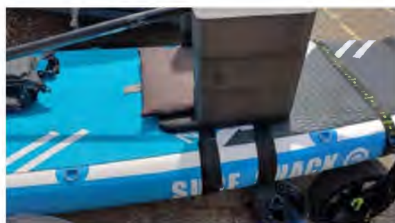
Prototype including the strapping, along with wheels to transport the board to the water
