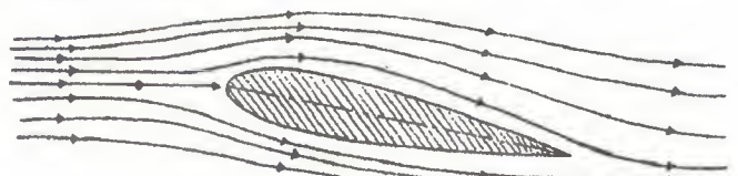
Flow Re-attaches Behind Separation Bubble
