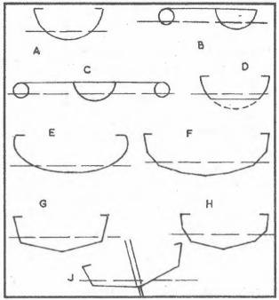
modern rigid and folding canoes and kayaks are close to this. With very few length-wise members, the result is called 'hardchine' (G) or 'double- chine' (H). These sections are now used for planked and plastic boats. Some Eskimo kayaks have these sections, probably because of a shortage of wood, rather than a knowl- edge of naval architecture.
