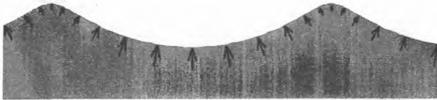
Shows combination at surface of acceleration due to wave motion and acceleration due to gravity for a wave of 6 metres wavelength, 1 metre height. Note that acceleration is always normal to water surface, and that acceleration is much less at the crest than in the trough.
