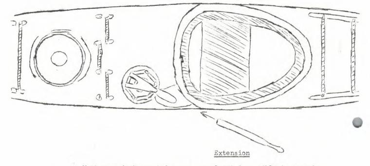
Most rear deck mounted pumps are almost impossible to operate when on the water due to being badly positioned. I've found an easy way to solve this problem is to use a slot on extension handle.
