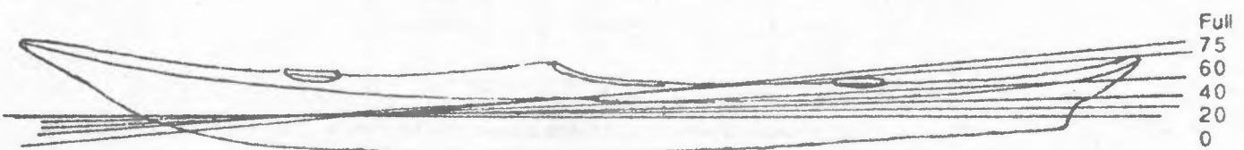
Water in Stern compartment
