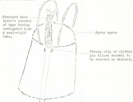
Place snorkel inside spray apron as shown. Gather top edge (only) of apron around tube and fasten with a clip. Tuck mouthpiece under a shoulder strap when not in use. We prefer to attach hull breathing devices to the spray apron rather than the kayak.
