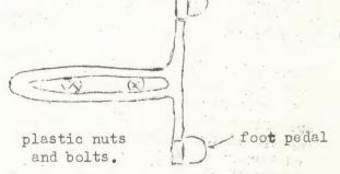
Control lines lie along the decklines to pass into the cockpit just forhead of the stern bulkhead. I use two foot pedals mounted to an adjustable 'T' piece. The rudder has made life so much easier, and I feel has lifted the safety factor for the boat. No worries about turning in strong winds.
