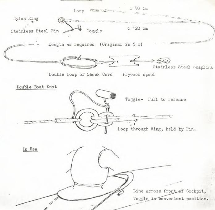
This towline system can be used on almost any boat, even a BAT. In the case of sea kayaks there is no interference with equipment on deck, although it could not be used on a boat with a rudder: The effective towing point is immediately behind the cockpit, where it should be, and the line can be released instantly if necessary. The cockpit rim forms a bollard, and the release mechanism with its toggle is in a convenient and readily found position at one side.
