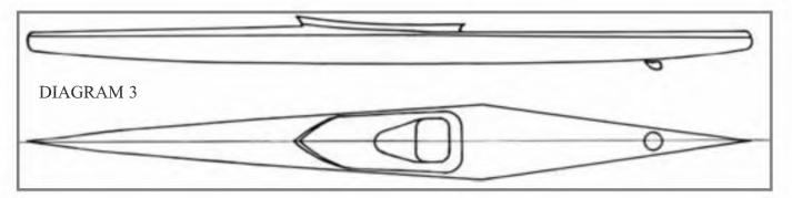
The less 'wetted' surface area of hull a kayak has, the less resistance there is from the water and the faster the kayak will be to paddle. The semi-
