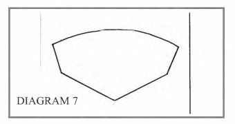
surface when paddled fast which makes them difficult to 'push' through the water. A 'soft-chined' hull i.e. one that has less abrupt angles at the chines, gives a smoother flow of water past the hull which reduces turbulence and so increases speed.
