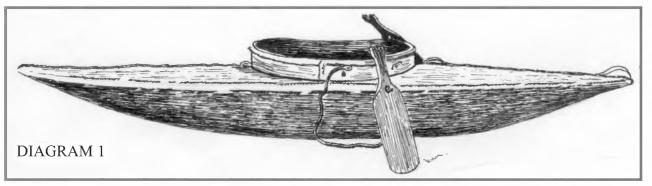
If a hull is highly rockered, i.e. has a marked curve from bow to stern, See diagram 1, it will turn easily. A strong sweep stroke on one side of the other will have the kayak spin easily. This is fine for
