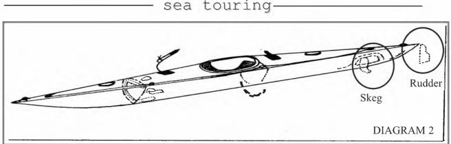
manoeuvring down slalom courses or for rock hopping in rough conditions. In the early days of modern Sea Kayaking most of us used this type of craft and we countered the rockered hull by fitting a skeg, of which more later. If the hull has little or no rocker the kayak will travel easily in a straight line and may even be difficult to turn, and hence may require a rudder or skeg. See diagram 2.
